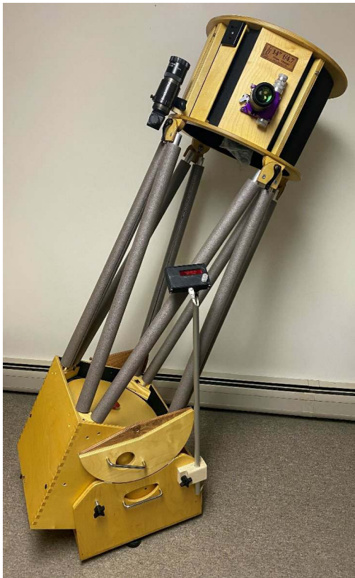
DIY Digital Setting Circle system attached to the VAS's 14"-Irene.
