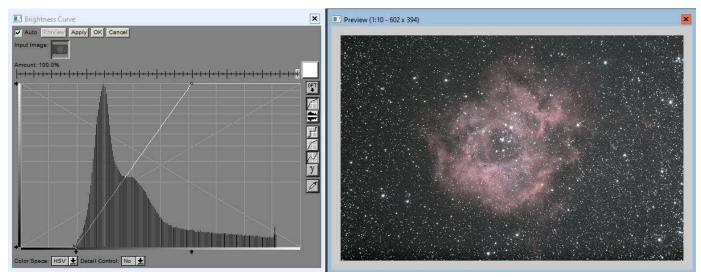
When the adjustment is applied the white diagonal line moves back to it's starting location between the lower left corner and the upper right corner "pulling" the pixel values with it, see below. Notice how the bumps in the graph are wider (stretched out) below compared to the graph above. If more "stretching" is needed, often it is best to apply the curve function a  $2^{nd}$  time.
