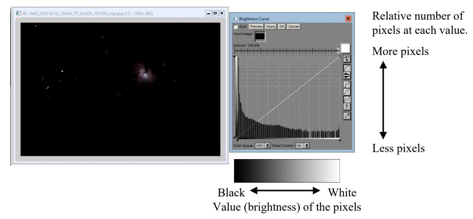
The **histogram or brightness curve**, is maybe one of the most useful tools available. It plots the number of pixels (vertical axis) against pixel brightness (horizontal axis). It takes some time to get used to looking at the data this way and using it to make adjustments to the image but is well worth the effort.
