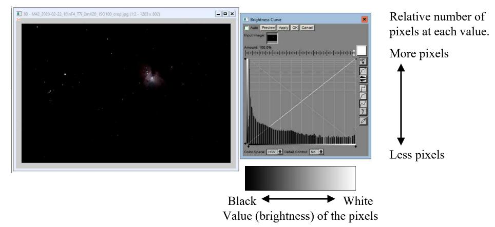
The histogram gives you a more accurate "picture" of the picture. Most of the pixels **are** very dark but not actually black. The nebula is represented by the vertical lines somewhere in the middle of the graph. The stars, by the lines on the right. Even an image like this with most of the pixels looking pure black has a lot of data hidden in all that blackness.
