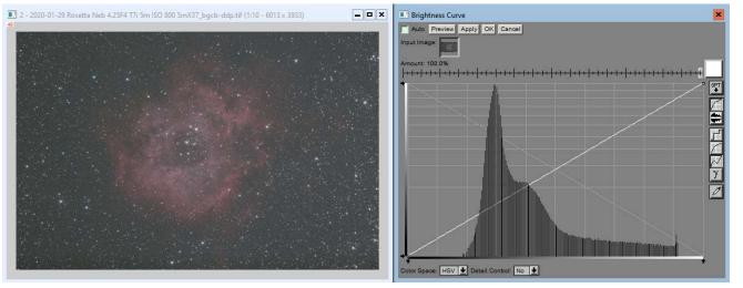
Here the background is too bright and the subject is not bright enough. With this particular software one uses the diagonal white line to make changes. Move the end points as shown below, the preview window on the right shows the effect.
