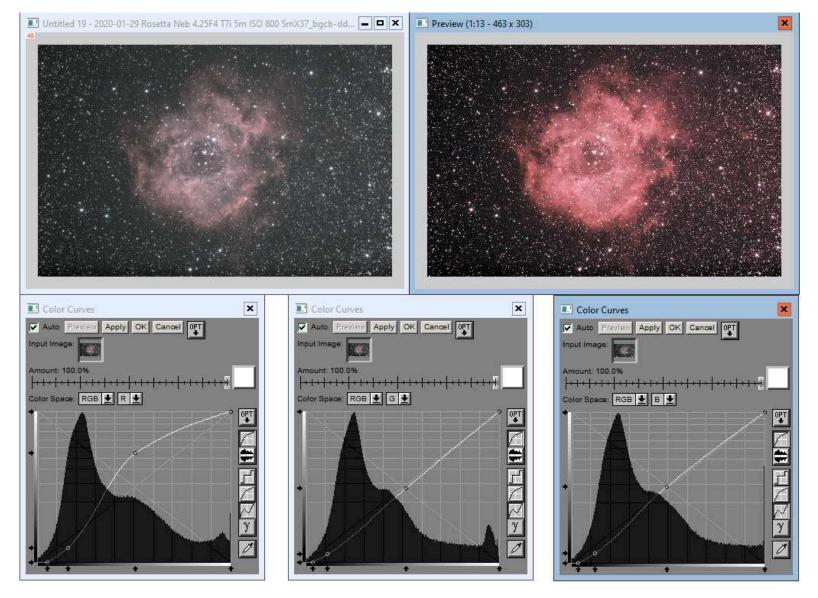
A more powerful tool is a color curve function. Here each color channel (red, green, blue) is adjusted independently. The red (left) brings out the H-alpha emission, here all 3 channels are used to darken the background.
