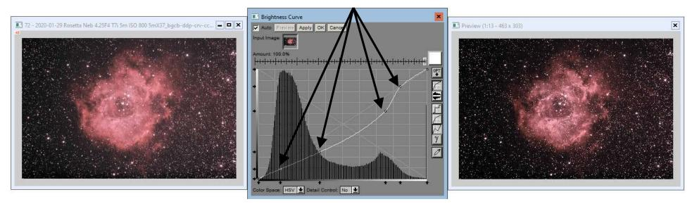
Here's another example of applying the curve function. This time to highlight details within the nebula. The curve or histogram function in some image processing software allows the user to place "grab points" as done here, giving the ability for complex and nuanced adjustments. Other's have very limited adjustments. Virtually all "post processing" functions manipulate the histogram of images in one way or another.
