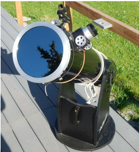
An Orion full aperture glass solar filter on an 8" Dobsonian Telescope.
